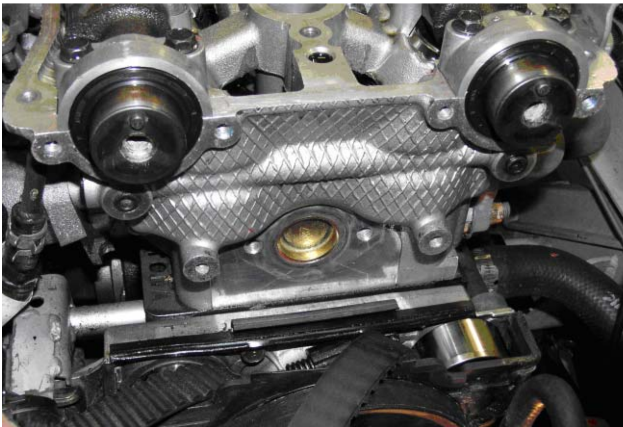
Figure 2 – Thermostat neck removed with new frost plug in place
