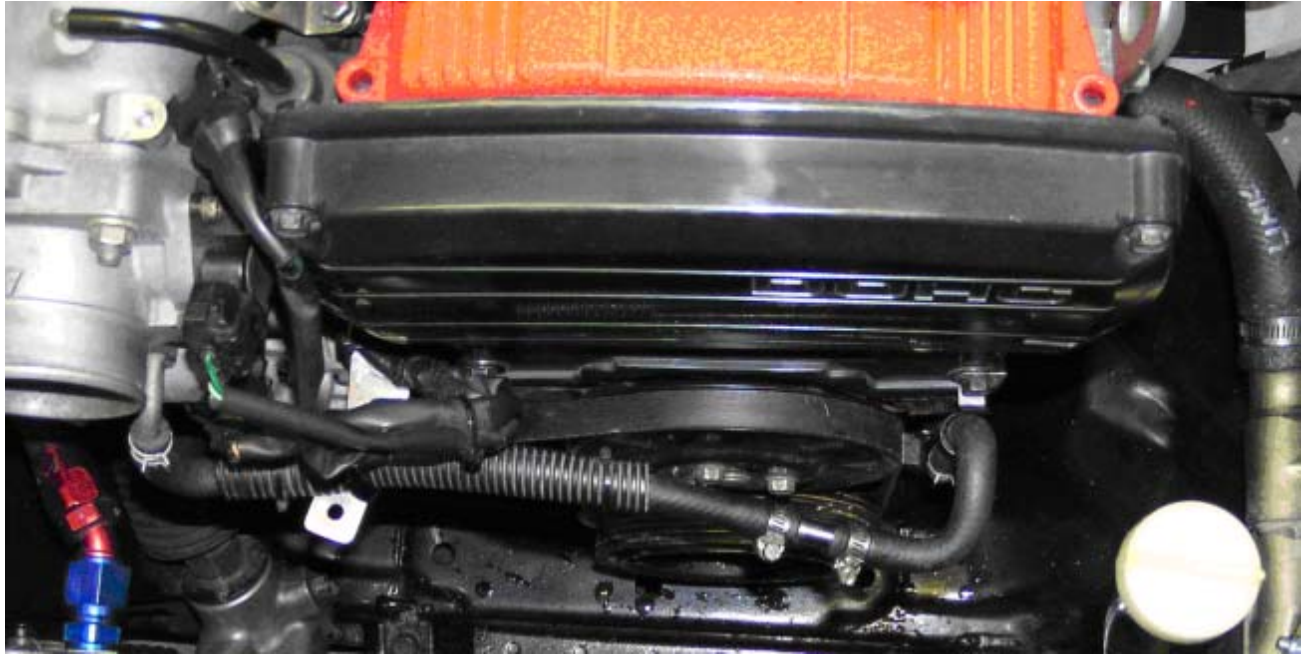
Figure 3 – Join in throttle body coolant feed
