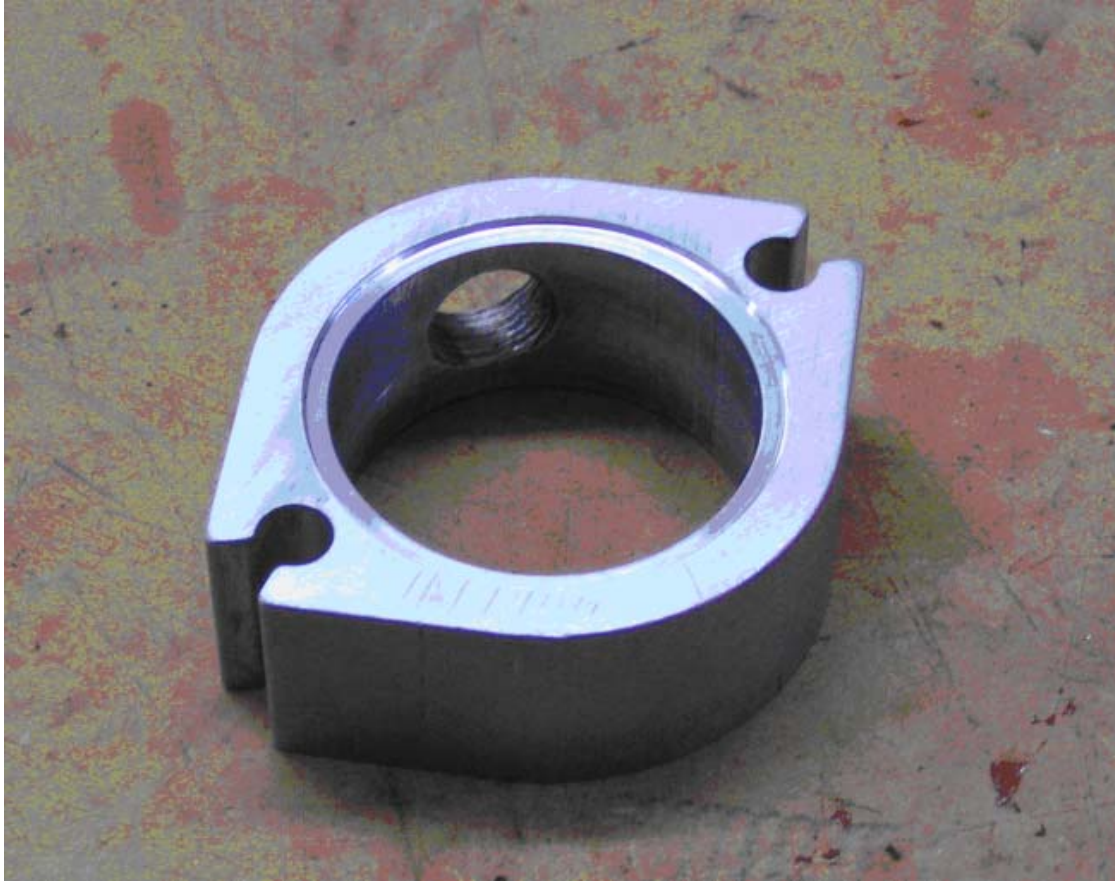
Figure 4 – Spacer block with thermostat rebate and 3/8 BSP thread
